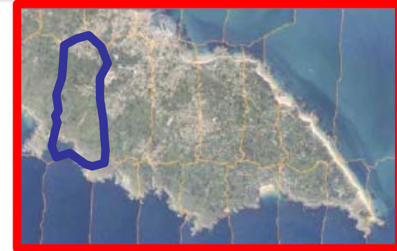
Figure 2 – mosaicked orthoimage with seamlines
